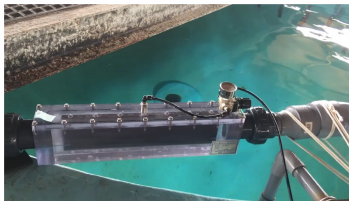
Figure 3: Anzii unit used for production of nano bubbles (photo: Morten Lykkegaard Christensen).
