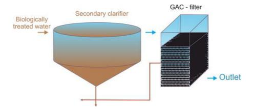
Figure 4. Schematic overview of the GAC unit suggested location in the conventional wastewater treatment technology (modified from<sup>15</sup>)
