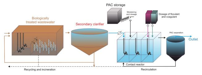
Figure 3. Schematic overview of the PAC unit suggested location in the conventional wastewater treatment technology (modified from<sup>14</sup>)
