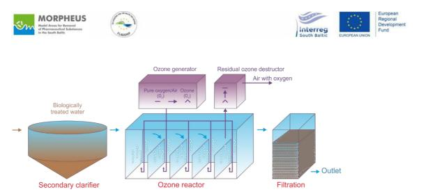
Figure 2. Schematic overview of the ozone unit suggested location in the conventional wastewater treatment technology (modified from<sup>13</sup>)
