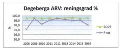
*Figure 2. Treatment efficiency of BOD*<sup>7</sup> *and P*<sub>tot</sub> *at Degeberga WWTP 2008-2016. Graph from Degeberga WWTP Environmental Report 2016.*
