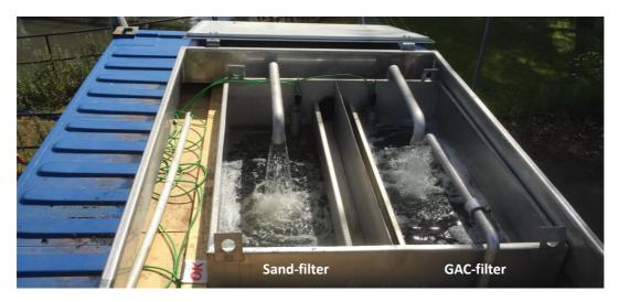
Figure 5. Pilot-scale plant in operation at a flow of  $2m^3/h$ . To the left 1  $m^3$  of sand as a pre-filter step followed by 1  $m^3$  GAC to the right. Photo: Erland Björklund.
