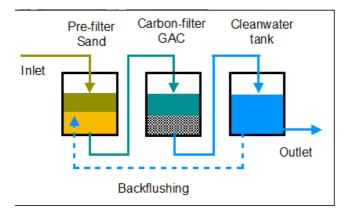
Figure 4. Design of the large pilot-scale treatment plant that was evaluated at Kristianstad Municipality with 50.000 m<sup>3</sup> waste water at a flow of 2m<sup>3</sup>/h, using a Triton® bottom filter for good throughput. The system consists of 2 filter units that can be connected serially or in parallel for increased flexibility, followed by a clean water tank. The pilot-scale plant was designed by Måns Hansson at Malmberg Water AB.
