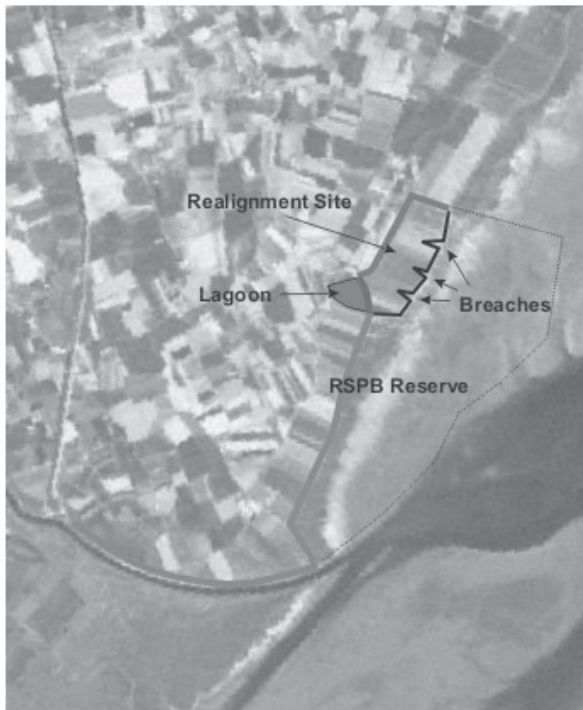
Fig. 5. A 'field scale' re-alignment along the Freiston Shore on the Wash. See http://www.thebostonwashbanks.com/ for further information.
