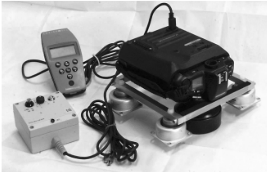
Fig. 1. The ADPS - Kodak Digital Science camera mounted on shock and vibration resistant chassis, Intervalometer and Trimble Ensign XL GPS receiver.
