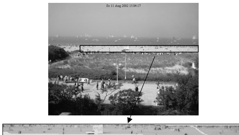
Figure 2: Example of a webcam image and the relevant beach area for the automatical survey (the white areas were masked out).
